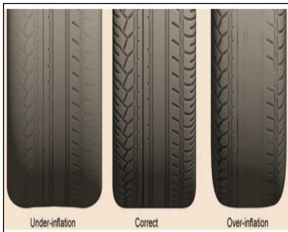
Fig.1.2: Tire wear patterns observed for different tire inflation pressures
